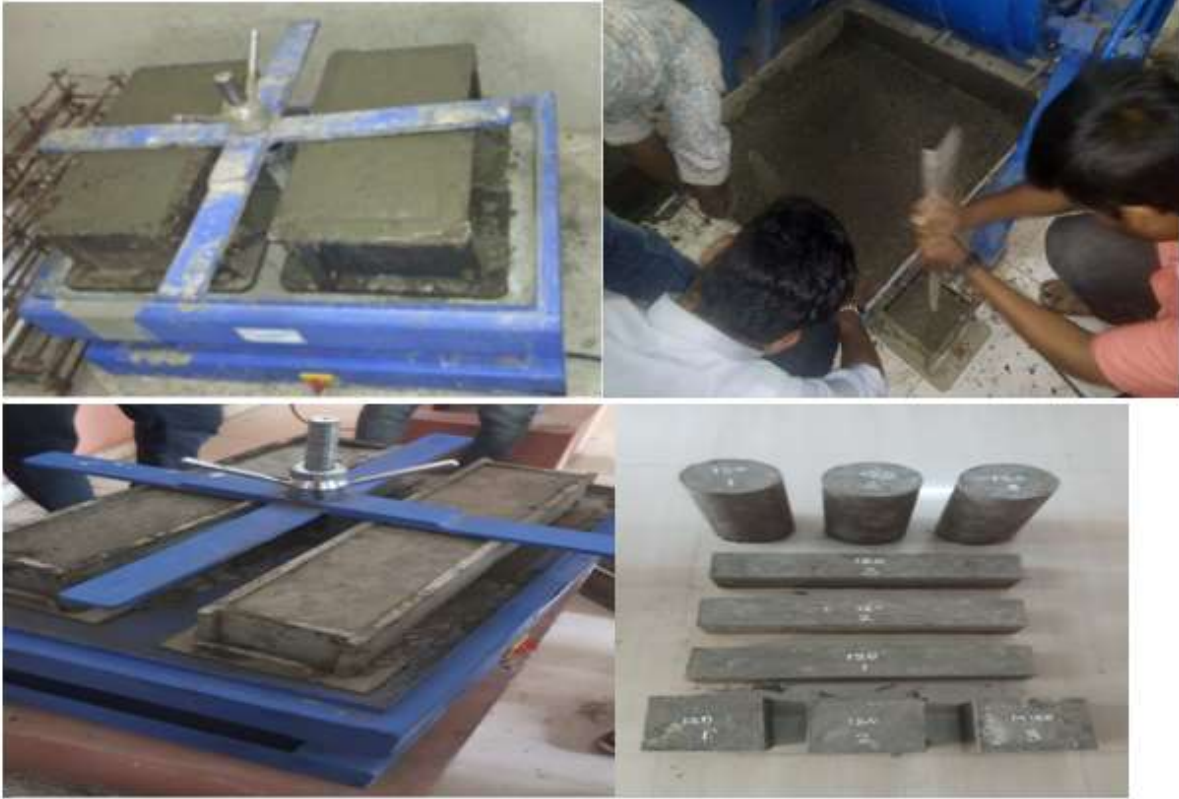
Fig 5 : Compaction of Concrete
