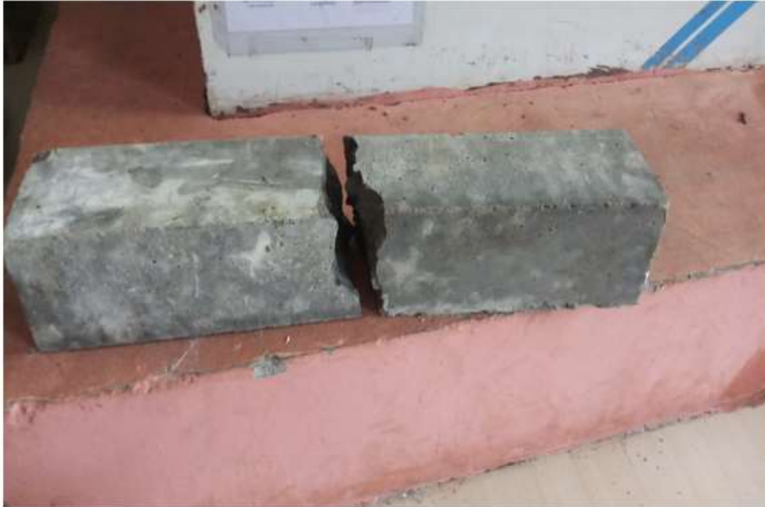
Fig 11 : Crack Pattern of Beams
