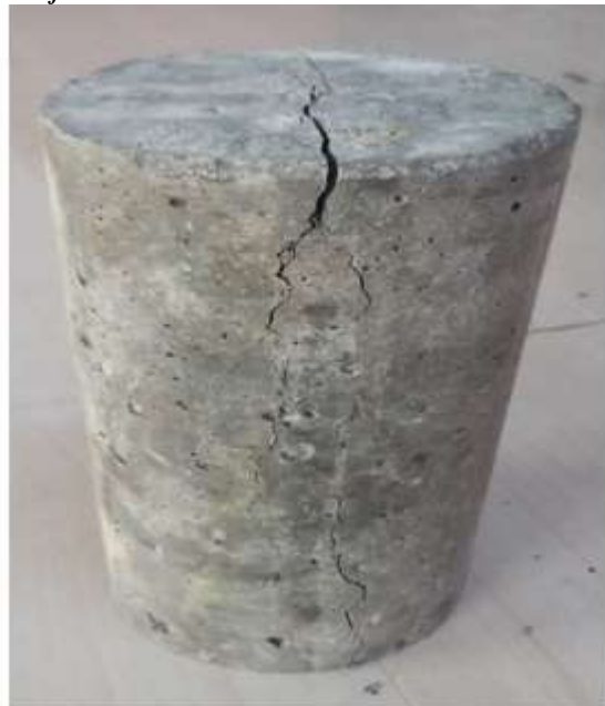
Fig 10 : Crack Pattern of Cylinders
