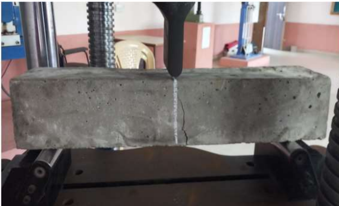
Fig 12 : Crack Pattern of Beams
